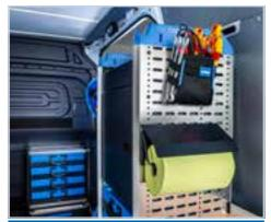
Flexible equipping of the aluminium side wall with accessories as required
