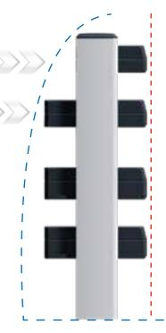
The reduction in component height at the top means that the components are still aligned in the direction of the middle of the vehicle. The advantage of this version is that the van racking system can still be used as a location for panel materials among other things. ProSafe lashing rails provide support surfaces and lashing options.
