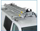
suitable for 1-, 2-, or 3-stage ladders; max. ladder length up to 1.5 times the length of the cross member spacing of the TopSystem; the cross member spacing can be varied from 1380 to 3000 mm up to 35 kg load
