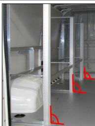
Arrange the block and the mounting parts parallel to the centre axis of the vehicle (1).
