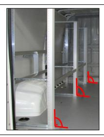
Arrange the block and the mounting parts parallel to the centre axis of the vehicle (1).
