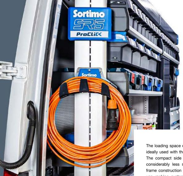
The loading space of the vehicle is ideally used with the SR5 concept. The compact side profiles require considerably less space than the frame construction of conventional van racking systems. In addition, ProClick is copatible with the side profiles so that tool bags or SR5 accessories can be hooked into the ProSafe perforations without using tools. Variation in the component depths and installation position means that the van racking system ideally adapts to the contour of the vehicle.
