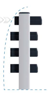
Installation of the components offset to the middle of the vehicle means that the SR5 shelving ideally adapts to the contour of the vehicle. The entire depth of the shelf is retained and the roof area in the vehicle is utilised to best advantage.
