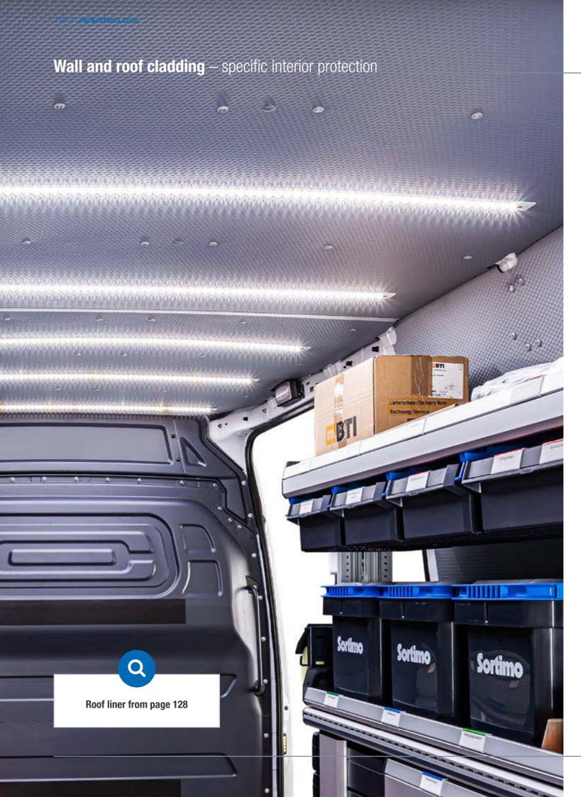
The SowaFlex wall and floor cladding, made from lightweight honeycomb material, protects the loading space of the vehicle and weighs 60% less than comparable wood cladding. The extremely impact- and scratch-resistant material protects the vehicle chassis in an optimum manner from damage and can be installed in the vehicle simply and without difficulty by fastening to the points provided by the vehicle manufacturer.
