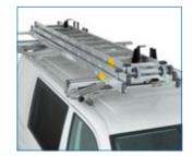
suitable for 1-, 2-, or 3-stage ladders; max. ladder length up to 1.5 times the length of the cross member spacing of the TopSystem; the cross member spacing can be varied from 1380 to 3000 mm
