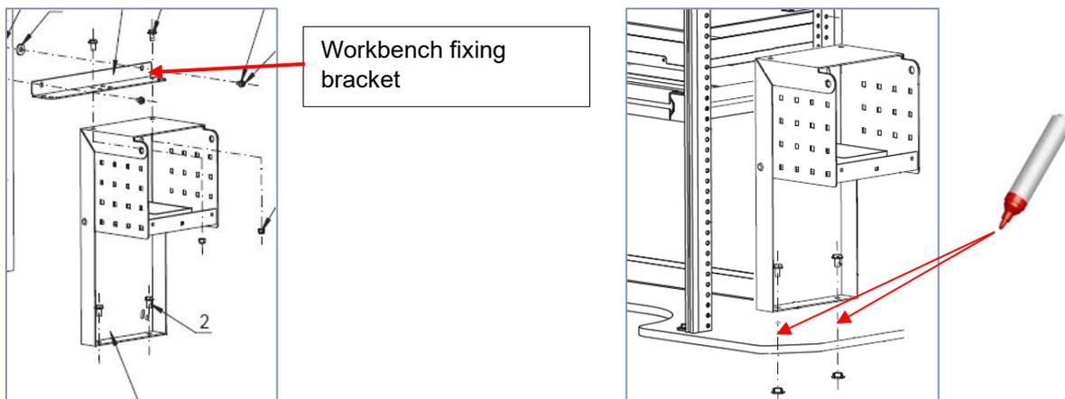
If the vehicle is equipped with side wall cladding, mark the attachment points on the side wall cladding.
