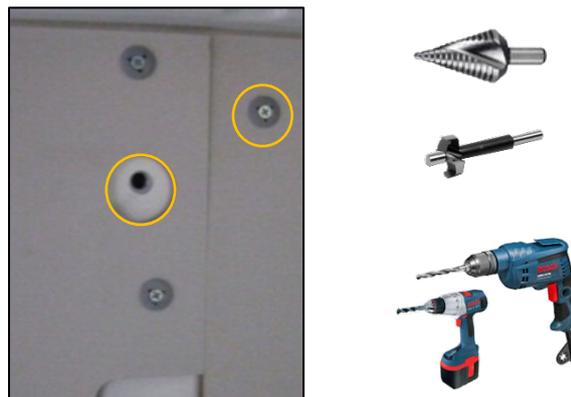
Depending on the fitting version, there are different ways of preparing the body of the vehicle for the final installation of the van racking system.
