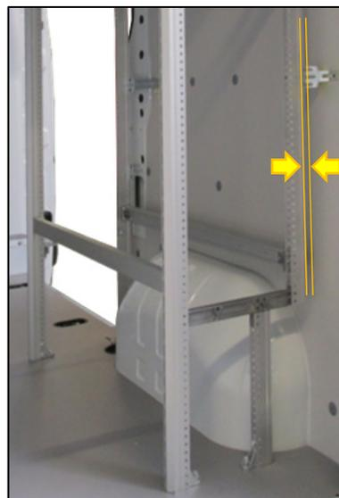
Level the block and mounting parts so that all connections are free of tension and the block is perpendicular to the floor.
