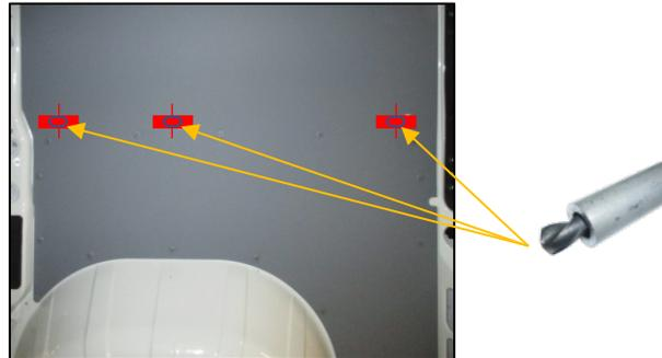
After this step, the side cladding can be removed from the vehicle.
