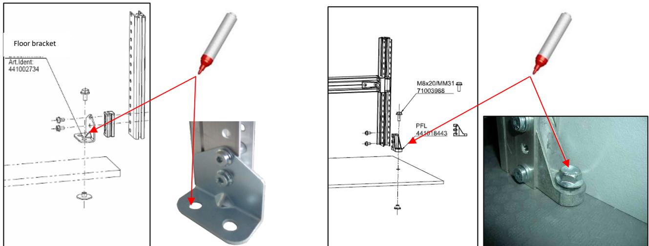
If a folding workbench is installed on the block, the drill holes also need to be marked here. The folding workbench bracket must be screwed hand-tight to the bracket of the workbench fixing.
